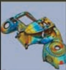
3D CAD Inspection - SLR Camera Cover
